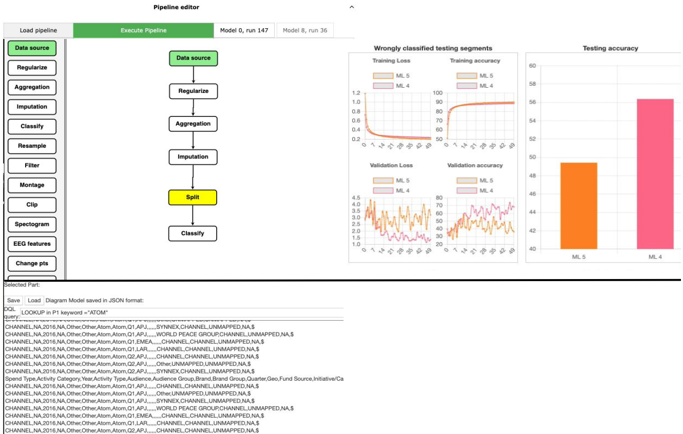
Figure 3: Dagger User Interface. Upper-left: Pipeline editor. Upper-right: ML performance charts. Bottom: Dagger console
